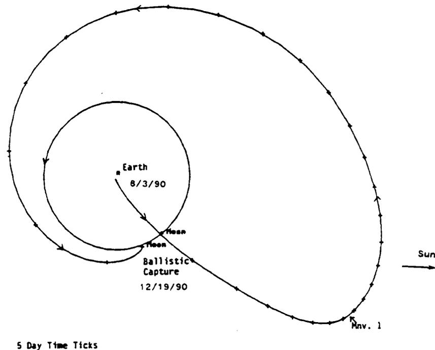
**Numerical simulation of a ballistic capture transfer trajectory for the Japanese spacecraft Hiten: ecliptic plane projection, sun's direction indicated at Earth injection.** (from Belbruno and Miller [1993])
