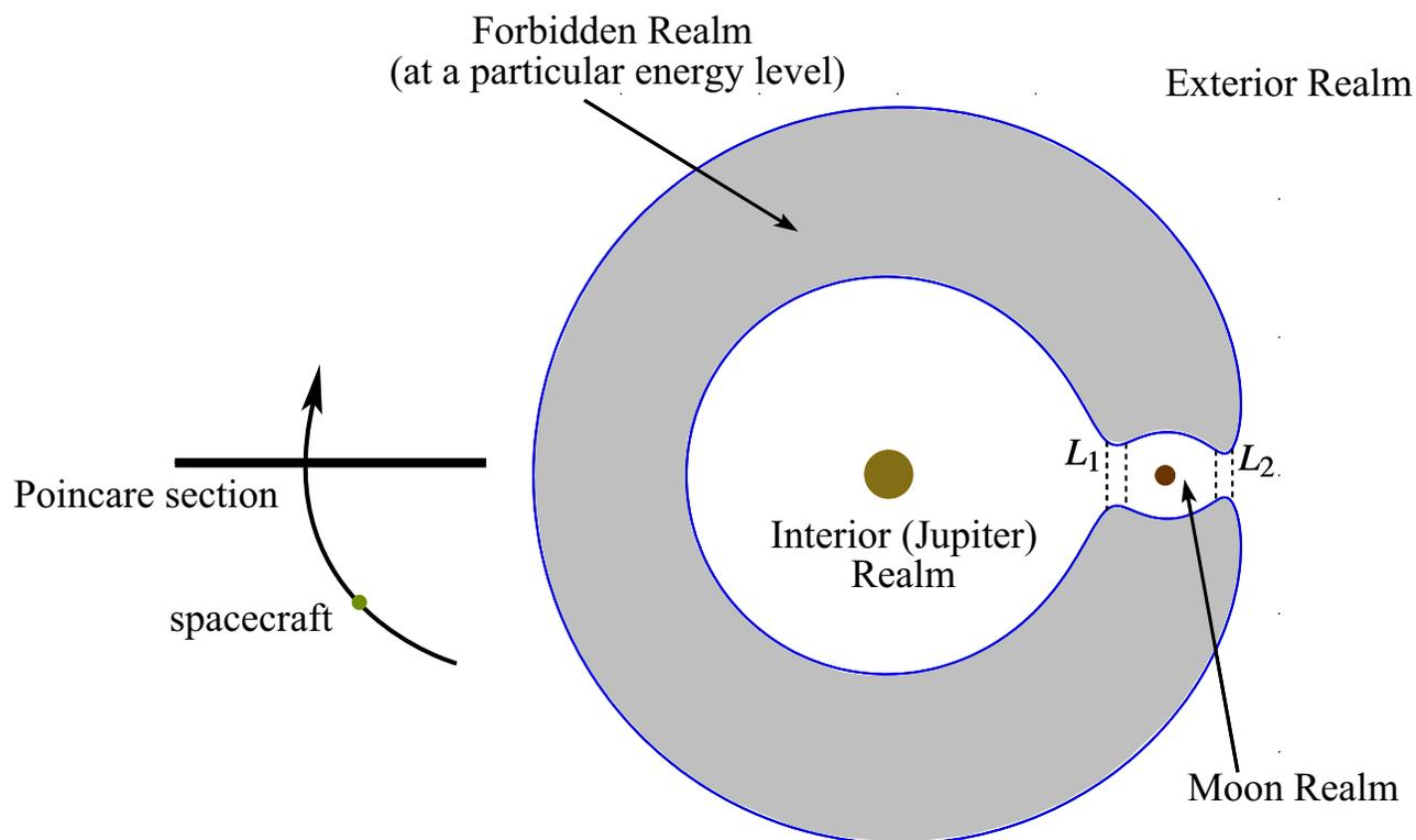
Rotating frame: different realms of motion at energy  $E$ .
