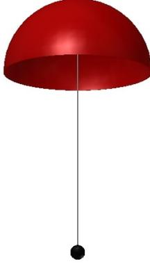
Figure 1: A more realistic parachute model. This model assumes a thin hemispherical shell plate as the canopy, a thin rod, massless rod connecting the canopy and the payload, and a spherical payload.
