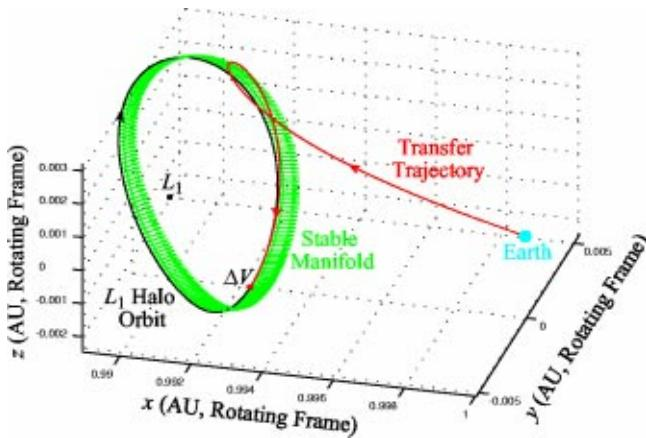
FIG. 43. (Color online) A transfer trajectory from low Earth orbit to an  $L_1$  halo orbit. This trajectory was constructed using the stable manifold of the halo orbit. The arrows attached to the halo orbit point in the direction of the stable manifold.
