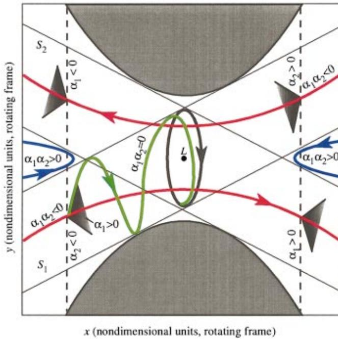
FIG. 9. (Color) The flow in the equilibrium region  $R$  of position space. Shown are the periodic orbit (black ellipse), a typical asymptotic orbit (green), two transit orbits (red), and two nontransit orbits (blue).
