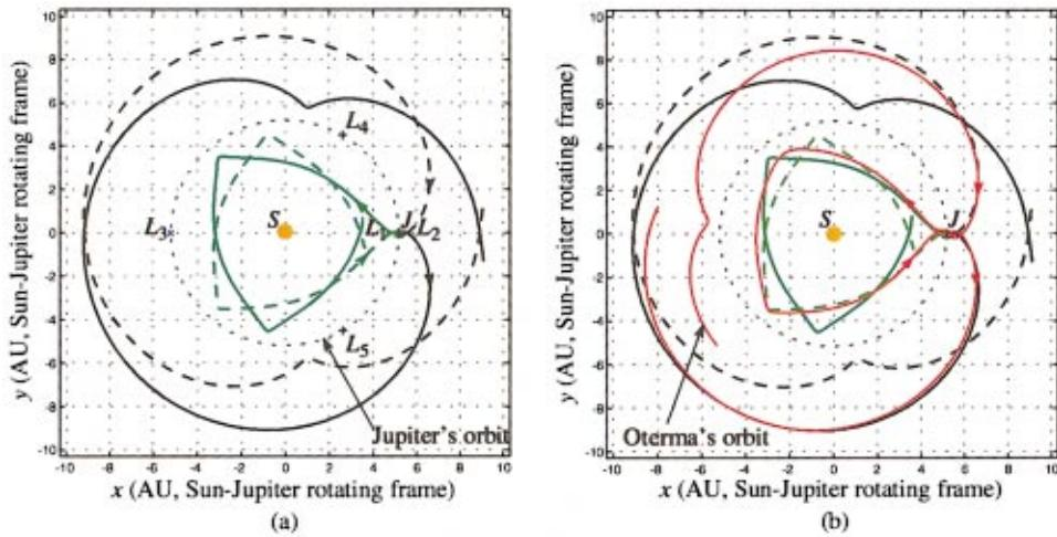
FIG. 1. (Color) (a) Stable (dashed curves) and unstable (solid curves) manifolds of  $L_1$  and  $L_2$  projected to position space in the Sun–Jupiter rotating frame. The  $L_1$  manifolds are green, while the  $L_2$  manifolds are black. (b) The orbit of comet Oterma (AD 1915–1980) in the Sun–Jupiter barycentered rotating frame (red) follows closely the invariant manifolds of  $L_1$  and  $L_2$ . Distances are in Astronomical Units (AU).
