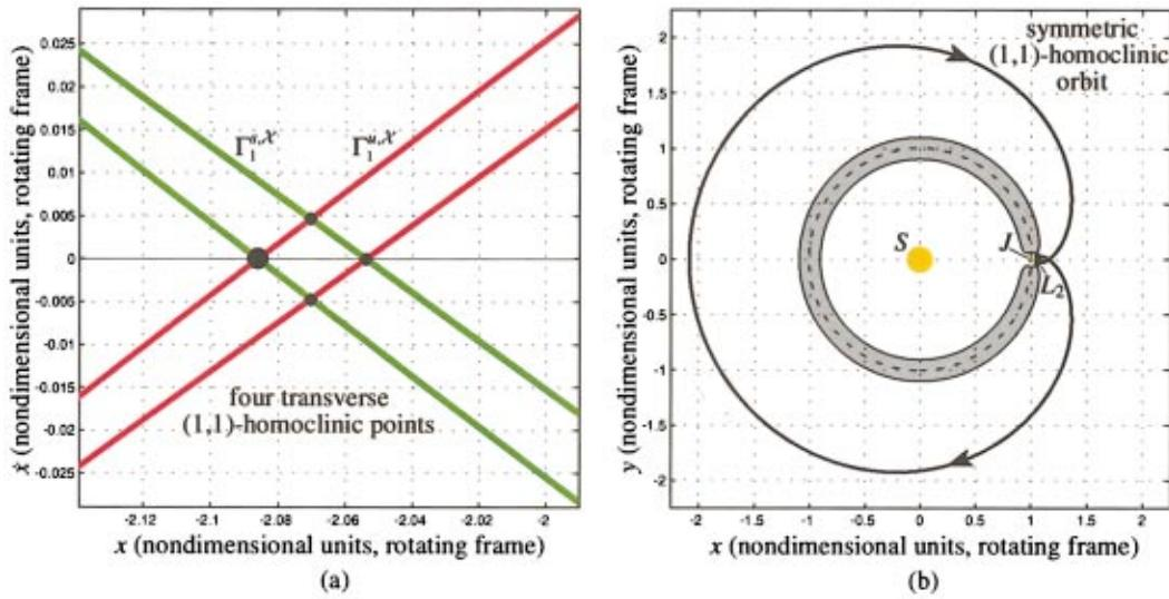
FIG. 19. (Color) (a) A group of four transverse (1,1)-homoclinic points. (b) The symmetric (1,1)-homoclinic orbit corresponding to the left  $\dot{x}=0$  (1,1)-homoclinic point [the large black dot in (a)].
