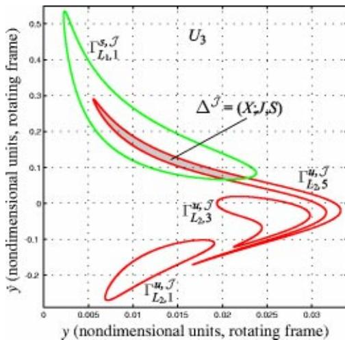
FIG. 33. (Color online) The first few transversal cuts of the  $L_1$  (stable) and  $L_2$  (unstable) Lyapunov orbit manifolds on the  $U_3$  section in the Jupiter region. Notice the intersection region, in which all orbits have the central block itinerary  $(X; J; S)$ .
