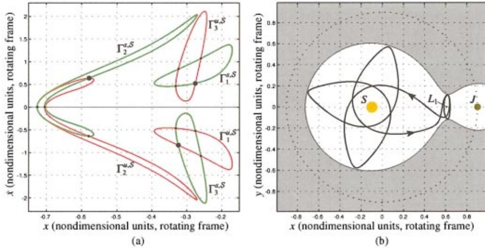
FIG. 21. (Color) (a) The first three Poincaré cuts of the unstable ( $W_{L_1,p.o.}^{u,S}$ ) and stable ( $W_{L_1,p.o.}^{s,S}$ ) manifolds with the plane  $y=0$ . (b) A nonsymmetric (1,3)-homoclinic orbit in the interior region [corresponding to the large dot in (a)].
