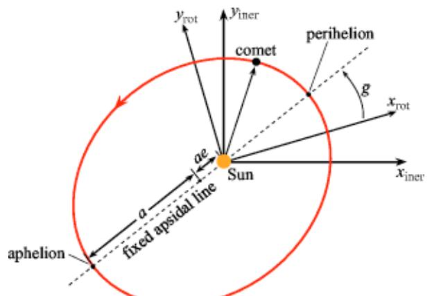
FIG. 38. (Color online) Geometry of the Delaunay variables. Elliptical orbits in the fixed (inertial) and rotating frames.
