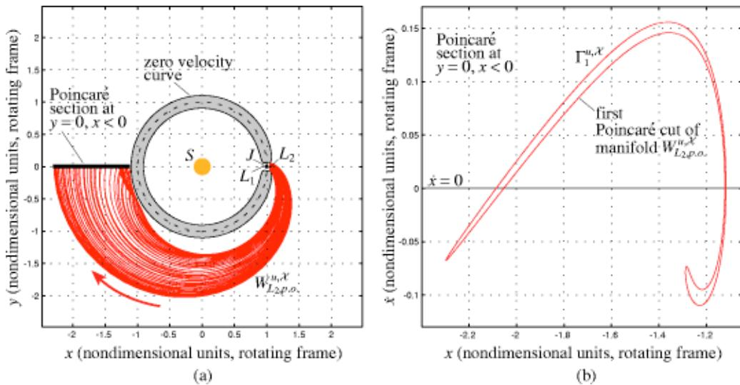
FIG. 18. (Color online) (a) The position space projection of the unstable manifold “tube”  $W_{L_2,p.o.}^{u,\mathcal{X}}$  until the first intersection with the Poincaré section at  $y=0, x<0$ . (b) The first Poincaré cut  $\Gamma_1^{u,\mathcal{X}}$  of the manifold  $W_{L_2,p.o.}^{u,\mathcal{X}}$  on the plane  $y=0, x<0$ .
