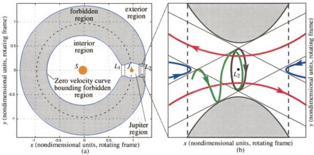
FIG. 5. (Color) (a) Hill’s region (schematic, the region in white), which contains a ‘‘neck’’ about  $L_1$  and  $L_2$ . (b) The flow in the region near  $L_2$ , showing a periodic orbit (black ellipse), a typical asymptotic orbit (green), two transit orbits (red), and two nontransit orbits (blue). A similar figure holds for the region around  $L_1$ .
