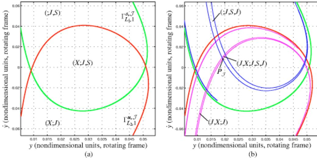
FIG. 41. (Color online) The Jupiter region  $U_3$  Poincaré section showing the image of  $\Delta^X$  (the 2:3 resonance portion) and the pre-image of  $\Delta^S$  (the 3:2 resonance). Notice their intersections, the largest of which is labeled  $(J,X;J,S,J)$ , corresponding to the itinerary of this group of orbits.
