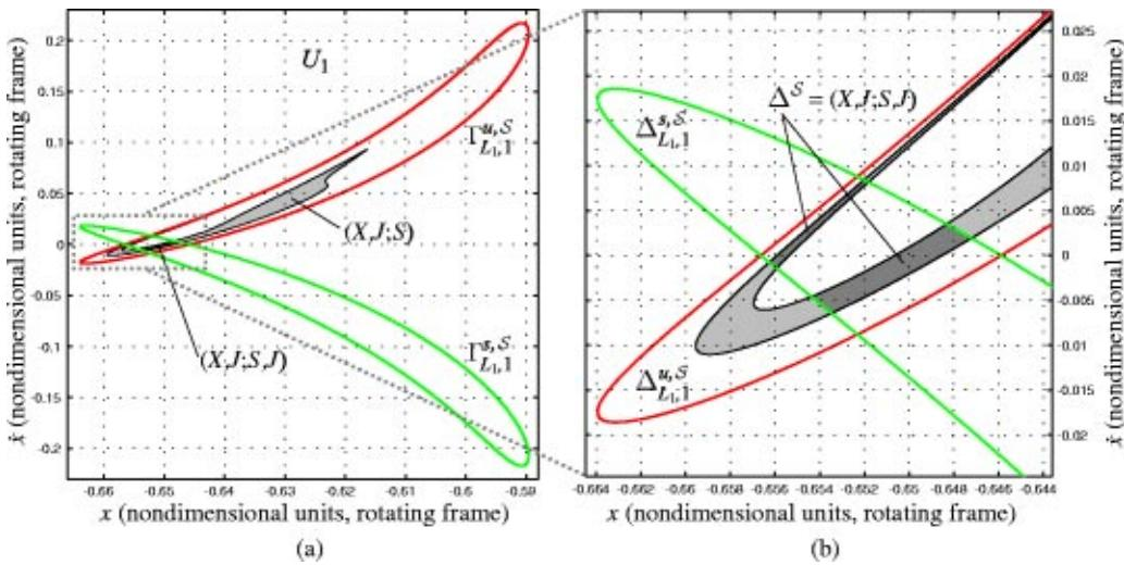
FIG. 34. (Color online) (a) Taking the  $(X;J;S)$  region of the  $U_3$  Poincaré section (see Fig. 33), we evolve it until it intersects the  $U_1$  Poincaré section in the interior region (lightly shaded). (b) A close-up of the intersection of the  $(X;J;S)$  region with the interior  $\Delta_{L_1,1}^{s,S}$  of  $\Gamma_{L_1,1}^{s,S}$ , the first stable manifold cut of the  $L_1$  Lyapunov orbit. Note the regions labeled  $(X;J;S;J)$ , which will return to the Jupiter region.
