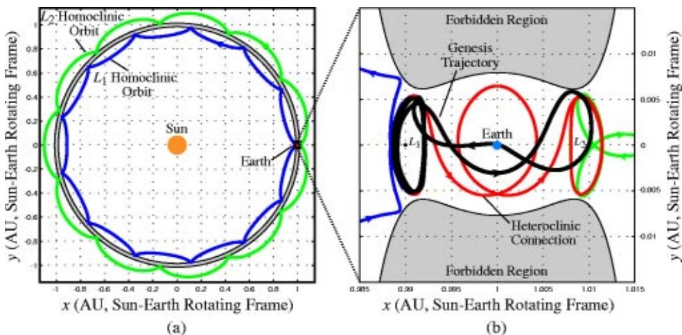
FIG. 42. (Color online) (a) A homoclinic-heteroclinic chain on the *Genesis Discovery Mission* trajectory's energy surface. (b) Close-up of the chain in Earth's vicinity. The actual *Genesis Discovery Mission* trajectory is shown in black overlaying the chain, and in particular, the heteroclinic connection from  $L_1$  to  $L_2$ .
