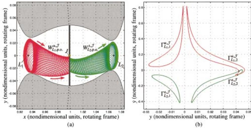
FIG. 22. (Color) (a) The projection of invariant manifolds  $W_{L_1,p.o.}^{\mu,J}$  and  $W_{L_2,p.o.}^{\mu,J}$  in the region  $J$  of the position space. (b) The first two Poincaré cuts of the invariant manifolds with the plane  $x = 1 - \mu$ .
