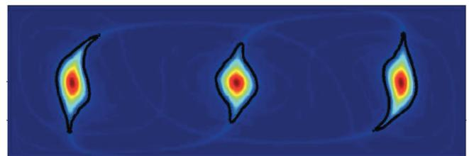
FIG. 7. AIS structure for  $\tau_f \approx 0.99$  based on  $v_2$ . The zero contour (black) is the boundary between the two almost invariant sets. Compare with the Poincaré section for the same  $\tau_f$  shown in Figure 4(d).
