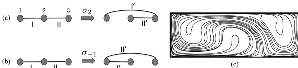
FIG. 2. The stretching of material lines under the action of the two generators in the reference case: (a) the action of  $\sigma_2$ , (b) the action of  $\sigma_{-1}$ , and (c) the actual stretching of a material line that is initially along the  $x$  axis in the reference case.
