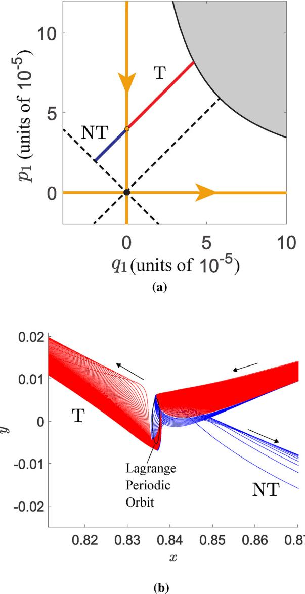
Fig. 9. (a) Numerically determined initial conditions for transit and non-transit orbits found by looking in the  $q_1$ - $p_1$  saddle canonical plane at initial phase  $\theta = 0$ .  $\tilde{H}_2 = 10^{-6}$  and  $c = 10^{-4}$ . Compare with schematic shown in Fig. 5. (b) The initial conditions integrated in the full equations of motion showing transit and non-transit behavior. Please refer to the online version of this article relating to color.
