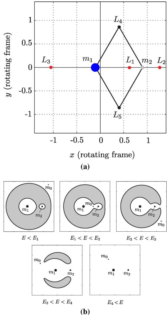
Fig. 3. (a) The Lagrange points of the CR3BP for  $\mu = 0.3$ . (b) The five cases of the energetically accessible regions (i.e., Hill's region) by CR3BP Hamiltonian energy.
