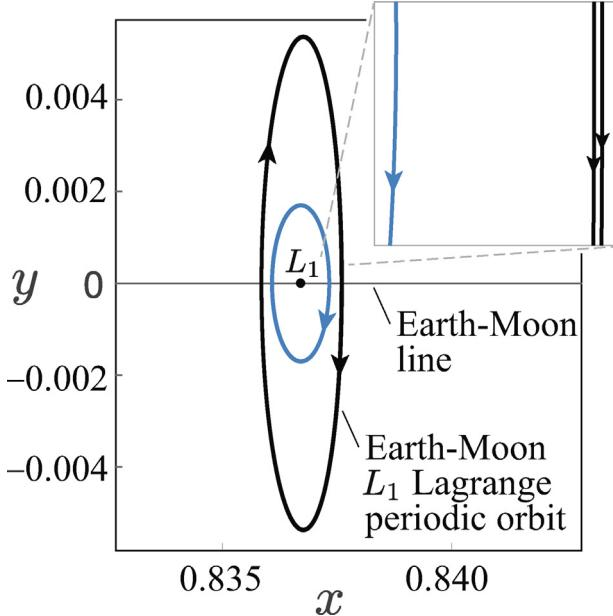
Fig. 8. The BCP Earth-Moon  $L_1$  periodic orbit (black) compared with the path (in blue) traced by the instantaneous zero, or stagnation point, of the BCP vector field. The former is a trajectory; the latter is not. Both have doubly-looping structures over a single period of the perturbation, but at the resolution shown, even in the inset, only the periodic orbit's two loops are visible.
