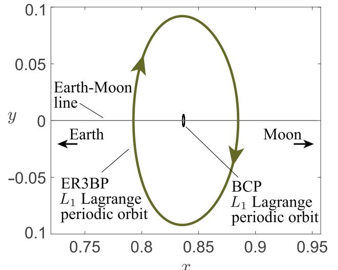
Fig. 11. The ER3BP Earth-Moon  $L_1$  periodic orbit (large, dark green) and the BCP  $L_1$  periodic orbit (black) in the position space (average rotating frame, CR3BP coordinates). The ER3BP  $L_1$  periodic orbit is singly-looping, not doubly-looping as in the BCP.
