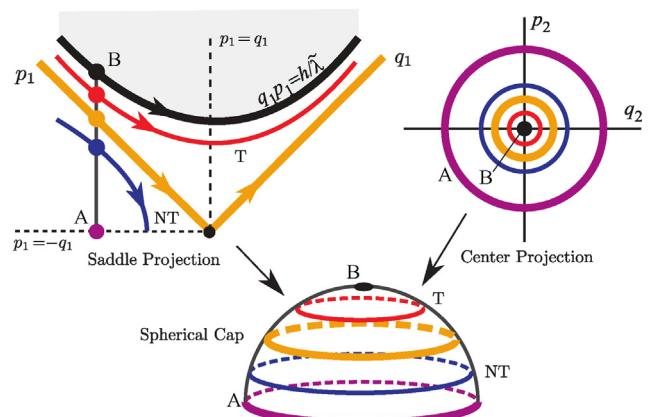
Fig. 6. Construction of a hemisphere bounding the equilibrium region of the map, along an energy manifold of energy  $h$ : each point along the bounding line AB in the saddle projection is associated with a circle of initial conditions in the center projection, shrinking to a point at B.
