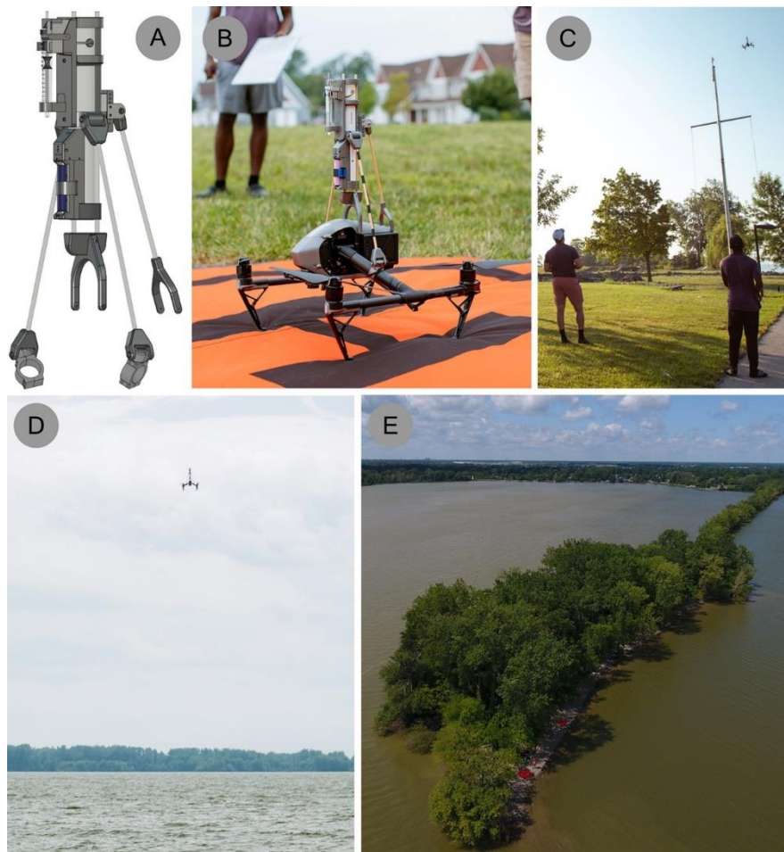
Figure 1. (A) Engineering model of the AirDROPS package. (B) The AirDROPS attached to the DJI Inspire 2 platform. (C) Intercomparison flight of the AirDROPS adjacent to the sonic anemometer mounted on the flagpole. (D) Sampling mission at GLMS, 10 m above the surface of the water. (E) Drone image and aerial view of the sampling location at LE to the right of the point in the image.
