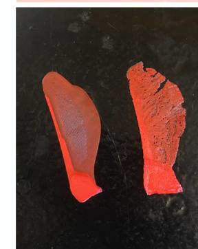
Left: A bioinspired maple seed (left) compared to a biomimetic maple seed (right). A more realistic looking seed that retains some of the critical characteristics for flight such as wing roughness and a slightly curved leading edge.
