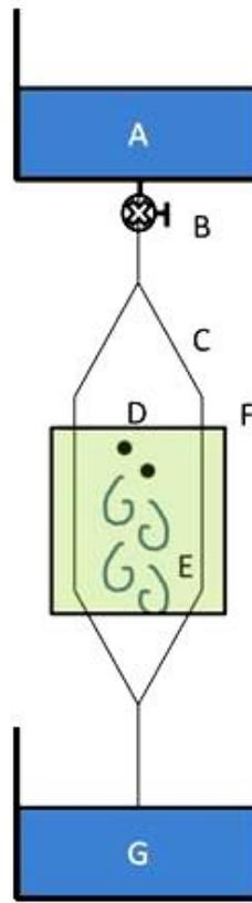
Figure 4: Conceptual diagram of the experiment setup. (A) Upper reservoir holding the soap water solution (B) Nozzle that controls the flow rate (C) Fishing line frame (D) 2 cylinders placed in the flow (E) Wake formation (F) Monochromatic light source (G) Lower collection reservoir.
