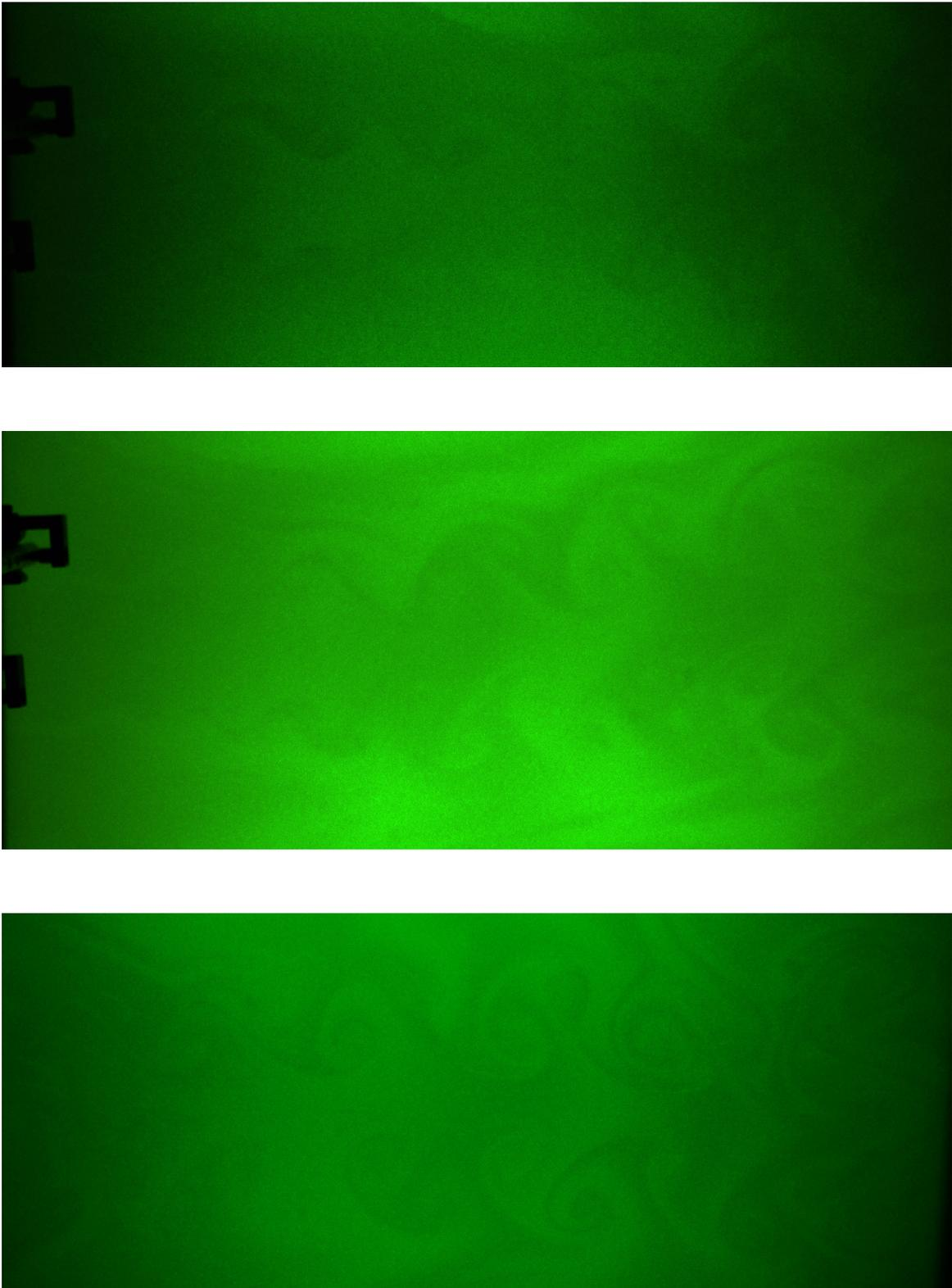
Figure 9: Sample snapshots of wake structures generated during our experiments. Two staggered cylinders operate as the bluff bodies. The test section has been illuminated by incident green monochromatic light from the rear. The central snapshot, for example, show the rough locations of the cylinders. They are held in place at the centers of the black projections.
