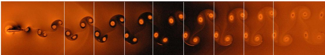
Figure 1: Typical 2P mode snapshot. A thin foil, which is imparted forced simple harmonic pitching oscillations, acts as the bluff body. The snapshot is from (2).
