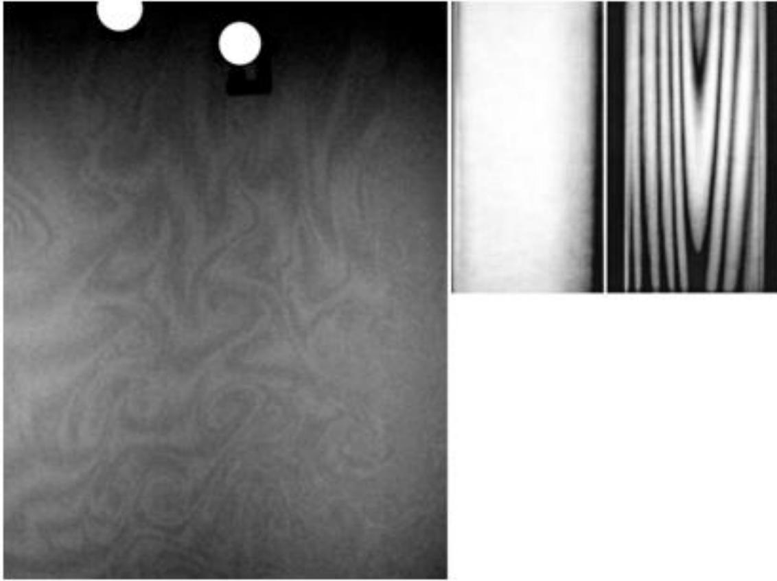
Figure 5: Wake visualizations. White circles highlight cylinder locations. Middle: Example of correct film thickness, Right: A film that is too thick (all the images are from (8)).
