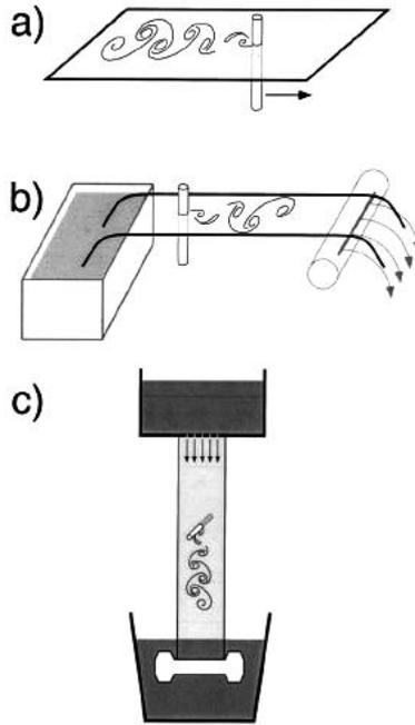
Figure 3: Employable methods of flow for soap film experiments (8).
